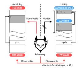
Fig. 1. Profiling of indirect code pointers by comparing Protected and Unprotected Execution States
